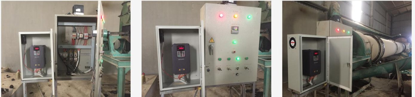
9- Inverter CT100 controls rotary turning kiln for fertilizer drying
