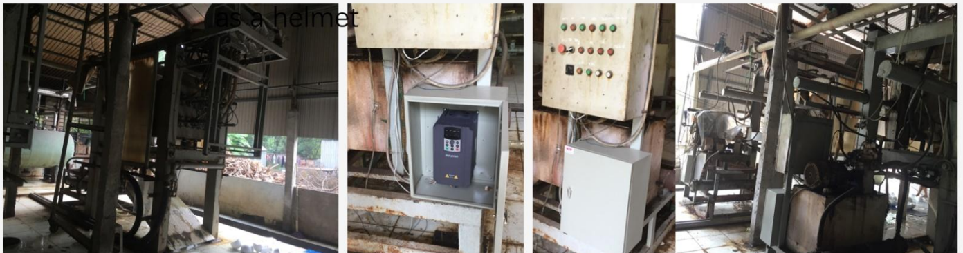
9- Inverter CT100 controls rotary turning kiln for fertilizer drying
